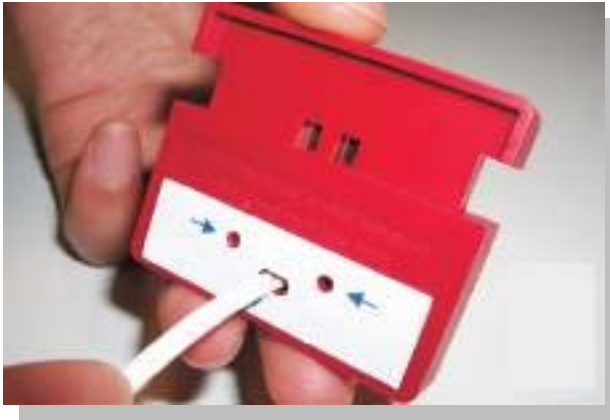
FIGURE 1 Slice the POF cable.
