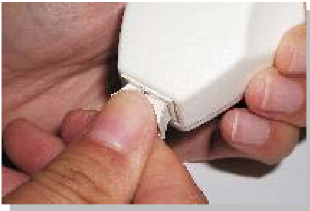
FIGURE 3 Insert POF into OptoLock.
